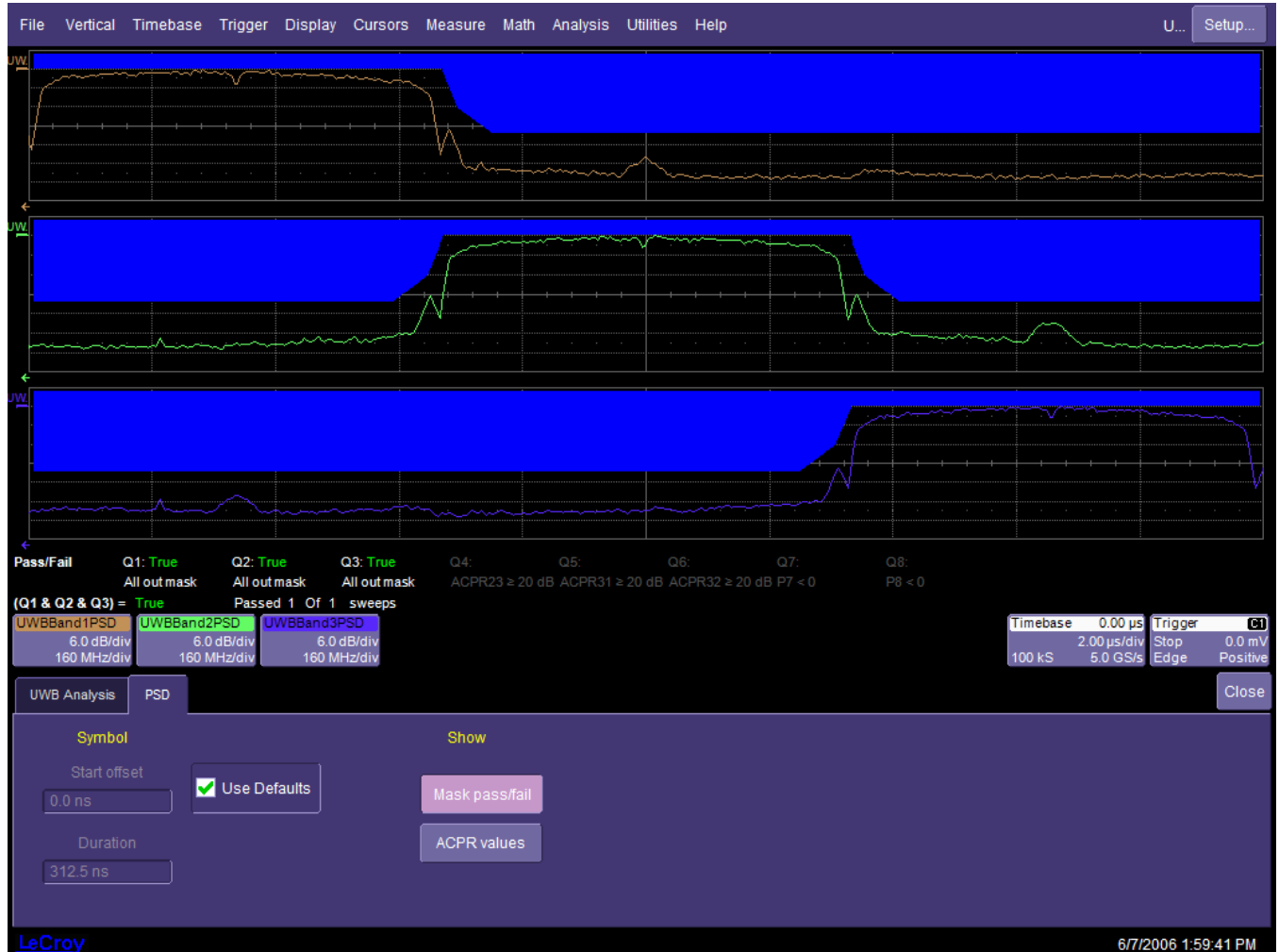
Example of the PSD Mask pass/fail testing view
